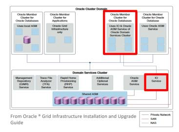
The I/O server instance receives data packets from the client and performs the appropriate IO to ASM disks
